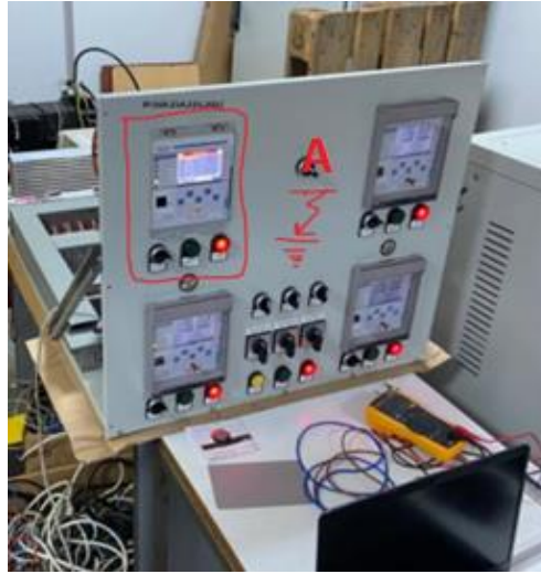
Figure 9. Directional relays in test system
