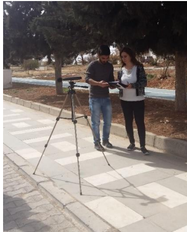
Figure 3. Noise measurement process and the Testo 861-1 noise measuring device
