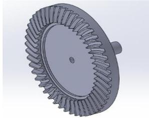
**Figure 5.** Ring gear view in Solidworks environment
