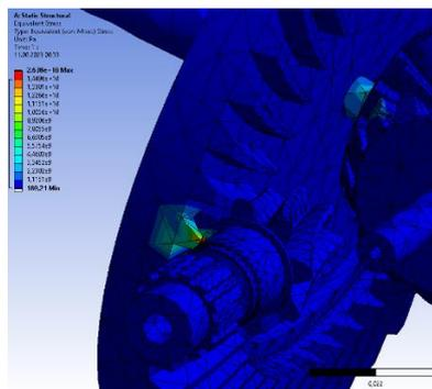
**Figure 8.** Stress analysis between ring and pinion
