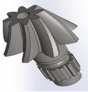
**Figure 4.** Pinion gear view in Solidworks environment
