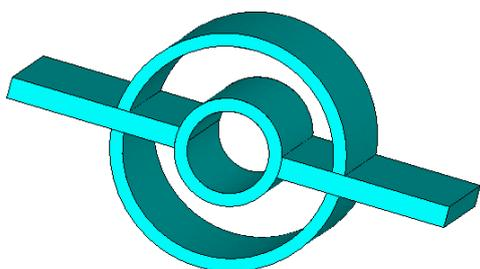
**Figure 18.** Energy absorbing member and fuse to control the buckling buckle
