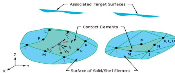
**Figure 4.** Contact elements 174 CONTA
