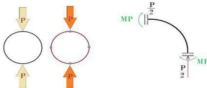
**Figure 2.** Formation of plastic joints in steel ring
