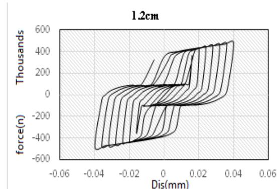
**Figure 11.** Curve of force and displacement for 1.2 cm
