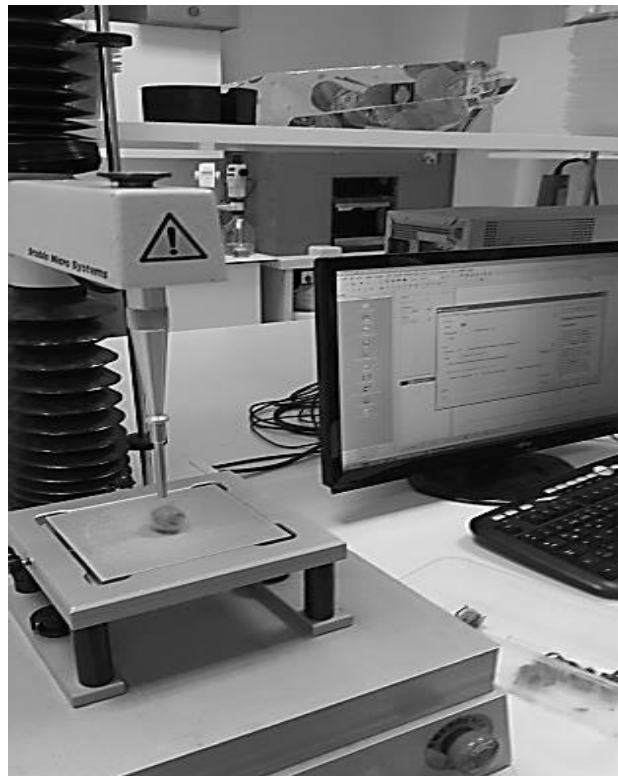
Figure 2. Texture analyses device
